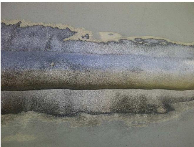
Detailed view of cleaned and roughened welding seam
