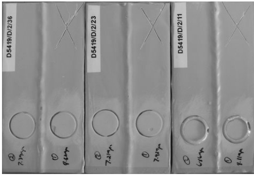
Figure 15: Sea water immersion 6 months no adhesion failure System 4 on any substrate
